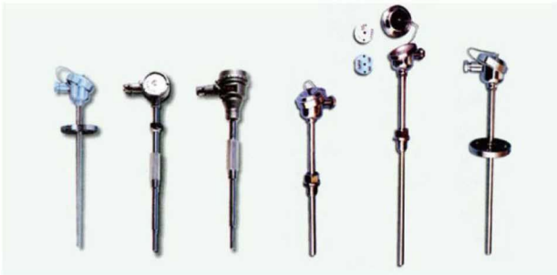
SHTR-07 Explosion-proof thermocouple and RTD series EMT/T graduation: K, N, E, J, T, S, R, B, Pt100, Cu50, Cu100 Junction box: Aluminium, Stainless steel Mounting option: Movable or fixed flange, Connecting thread Flange standard: GB, HG, JB, HGJ, SH, ASMEB, ANSI, JIS Armored element: Simplex or duplex
