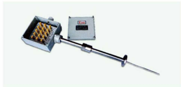
SHTR-12 Multi-point armored thermocouples For petroleum, petrochemical, gas, metallurgy industrial fields. Single multi-point: Most points 6pcs, Max length 8m Multiple multi-point: Most points 30pcs, Max length 150m Protection class: General-sheathed or explosion-proof
