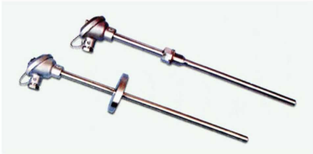
SHTR-09 Water-proof thermocouple and RTD series EMT/T graduation: K, E, J, Cu50, Pt100 etc. Junction box: Stainless steel Mounting option: Fixed flange, Connecting thread Flange standard: GB, HG, JB, HGJ, SH, ASMEB, ANSI, JIS Armored element: Simplex or duplex
