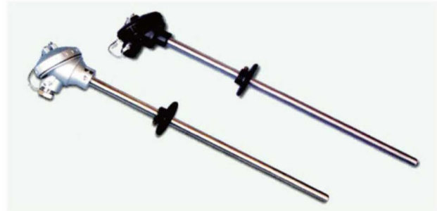
SHTR-10 Movable flange thermocouple & RTD EMT/T graduation: K, E, J, T, Cu50, Pt100 etc. Junction box: Black plastic, Aluminium Mounting option: Fixed flange, Connecting thread Armored element: Simplex or duplex
