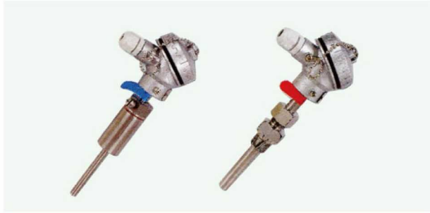
SHTR-01 Paired Temperature Sensors for Heating System With big Junction box, G1/2" stainless steel Resistor type: Pt100, Pt500, Pt1000, class A, class B Range: 0-135°C standard, 0-400°C available Connection: Sliding connection, fixed connection with tube
