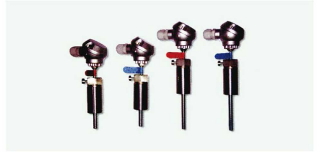
SHTR-02 Paired Temperature Sensors for Heating System With small Junction box, G1/2" stainless steel Resistor type: Pt100, Pt500, Pt1000, class A, class B Range: 0-135°C standard, 0-400°C available Connection: Sliding connection, fixed connection with tube
