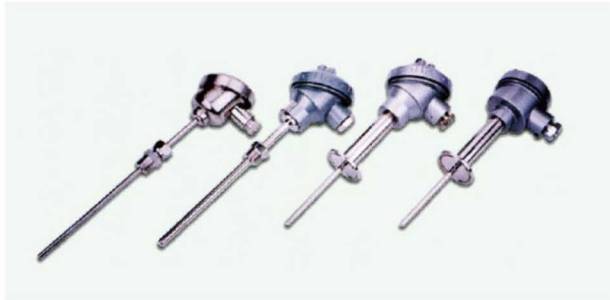
SHTR-03 Thermocouple and RTD Used for food, dairy, beverage, medicine, and chemical industries. Stem OD 1/4"(Φ6.35), L=2.5", 4", 6" etc. Option: Material and connection of socket and stem
