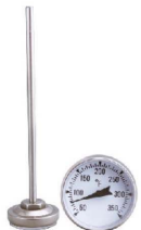
NO.: SH-B1M Dial/Size : \Phi 26 mm Stem Size: \Phi 3.8 \times 116 mm Main material: Stainless steel 304
